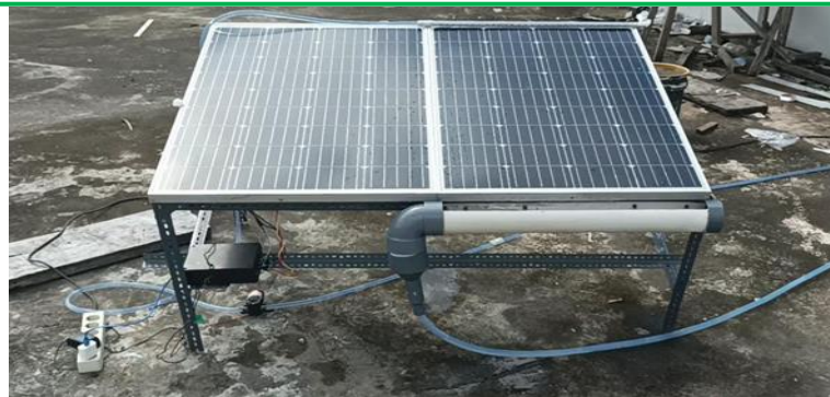
Gambar 2. Water Cooling System (WCS)
